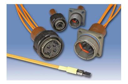
Amphenol D38999 connectors can be supplied with inserts that accommodate MT optical ferrules. This combination offers a high fiber density in a relatively small cylindrical connector package with all the advantages of the MIL-DTL-38999 Series III proven connector.
