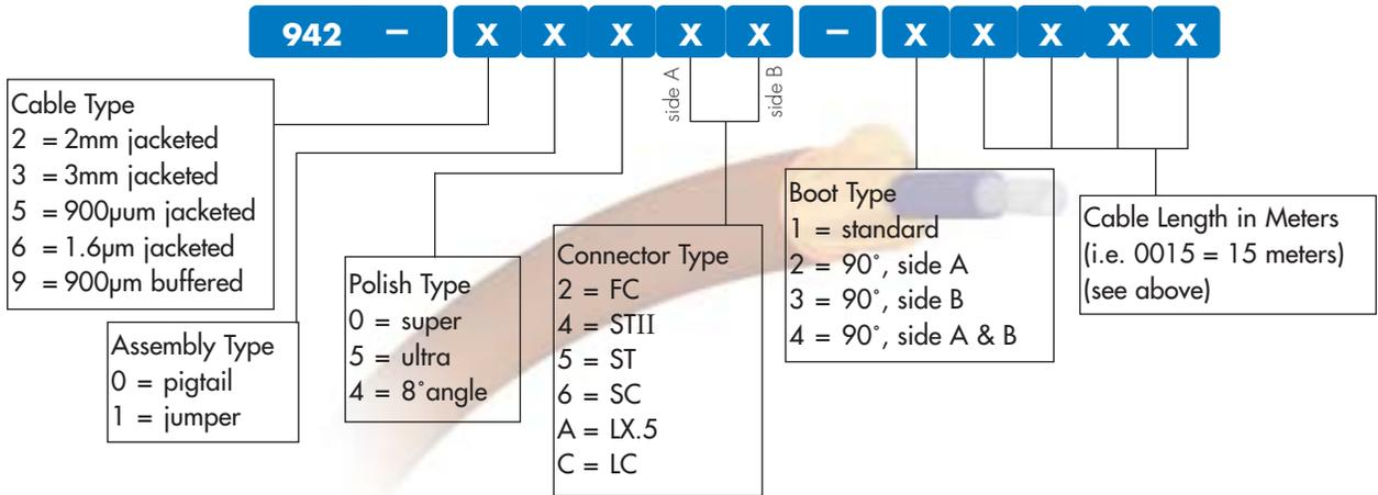
Note: For pigtailed, connector type side A and side B are identical (i.e. SC pigtail: connector type = 66).
