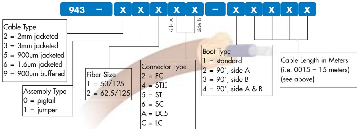
Note: For pigtail, connector type side A and B are identical (i.e. SC pigtail: connector type = 66).
